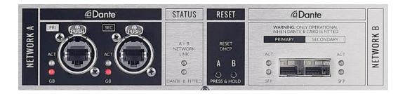
A16.D16 has two redundant sets of network connections. The Network A ports feature etherCON ruggedised RJ45 connectors. The Network B ports are SFP cages which can be fitted with either RJ45, single-mode or multi-mode LC fibre connectors. This connectivity would require an additional Dante card which is not currently available.
