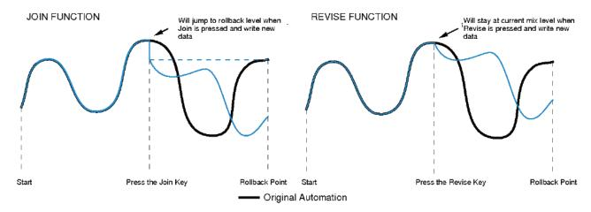
Multiple Rollback memories are supported so that successive operations of Join or Revise return different sets of faders back to the write state, if multiple Rollback operations have taken place.
