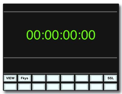
**VIEW** is selected automatically by the **GLOBAL** key to access the eight Global View select keys. It can also be selected manually if required. There are no tallies for the selected view. **VIEW** is an AWS function and not part of the MCU protocol.
