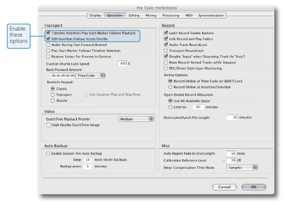
Enable the two options circled above. This ensures that the MMC locate messages are transmitted correctly from Pro Tools.
