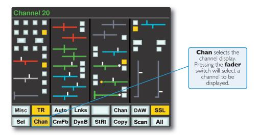
The large switch above each fader (bottom right-hand corner) refers to the status of the channel's cut button, and the smaller switch refers to the solo-isolate function.
