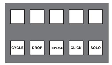
Only five of the ten keys above the Motion controls are assigned. These have on screen tallies in the status area of the TFT display.
