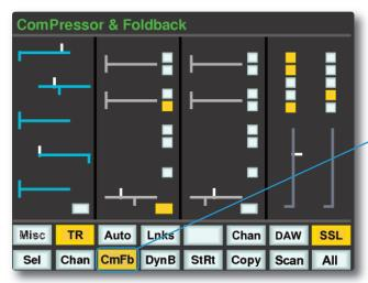
Pressing **CmFb** or pressing the master fader switch will display the centre section compressor, the master fader and foldback sections. A double press on the fader switch will reset the REC and MIX fader positions and the REC and MIX processing switches.
