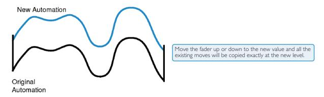
Both Autotakeover and Snap functions (see below) used in conjunction with a Trim update allows a seamless or smooth return to the stored mix data.
