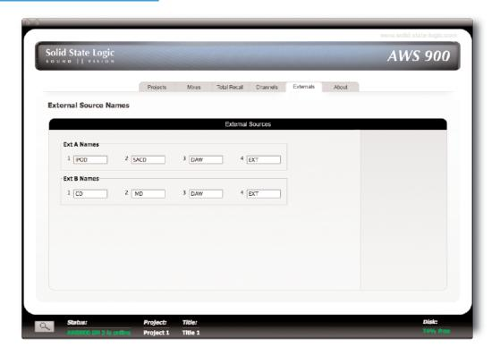
The **Externals** tab allows you to rename the External sources (Ext A + Ext B). These will appear on your console's monitor section.
