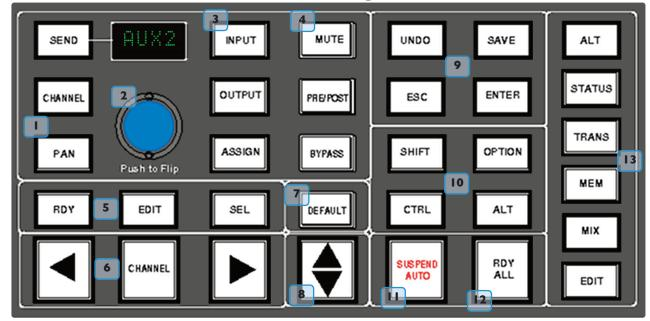
The function of the channel **SEL** ( 17 ) button depends on the mode selected on the centre section **RDY**, **EDIT** and **SEL** keys on the Master Control Panel.
