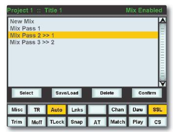
New Mix Passes are auto-numbered starting at '1'. If a Mix Pass is deleted (see below) then its number will not be re-used. The only exception to this is if all Mix Passes are deleted. The numbering will then restart from '1'. Mix Passes can be renamed from the AWS Remote — see Renaming Mix Passes.
