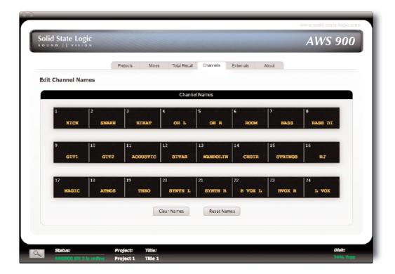
The **Channels** tab allows you to enter names for the AWS console channel scribble strips.
