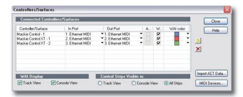
Once the MIDI ports are configured, select the Mackie Control device from Sonar's Tools menu to open the Mackie Control properties page, and use the Configure Layout feature to map the AWS channels to the Sonar mixer channels using the AWS channel V-pots, as prompted on the channel scribble strip displays (note: the AWS must be in DAW focus mode).
