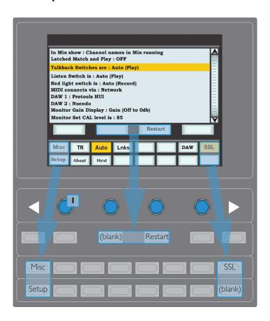
To change a setting, use the left hand V-pot ( ) to select the item, then press the V-pot to enter adjustment mode. Turn the V-pot to the desired setting and press it a second time to save the setting.
