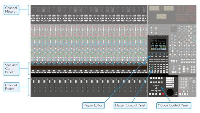
The AWS faders and Solos and Cuts panels can be switched between controlling the analogue audio signal path and the DAW using the Focus switch – see below. The Motion Control Panel, Master Control Panel and Plug-in Editor always control the DAW. The illustration above shows the DAW controller elements in 'DAW Focus Mode'. The greyed-out areas indicate analogue-only console elements.
