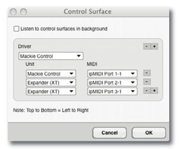
Assign the AWS MIDI ports so that the console faders map correctly to the DAW tracks with the Mackie Control Unit as channels 17-24.
