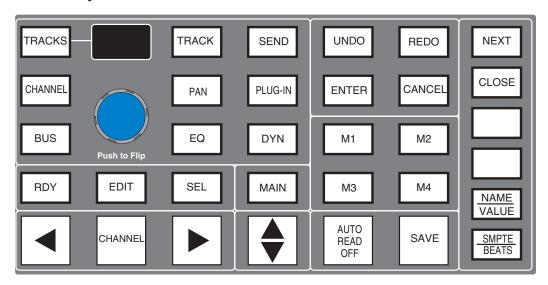
The majority of functions are controlled via dedicated keys with less reliance on the 8x8 key matrix located beneath the screen than with the HUI version.
