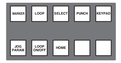
Tallies are shown in the status area of the TFT display for Loop ON/OFF, Jog Parameter, together with tallies for Marker, Loop, Select and Punch. As the later functions intercancel, they share the same on screen area.
