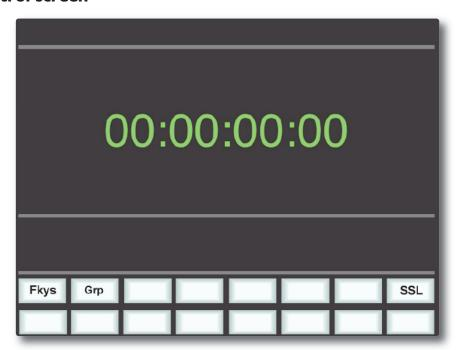
Fkys are the eight functions keys. These are also mapped to the numeric keypad, which is not supported in Logic Control.
