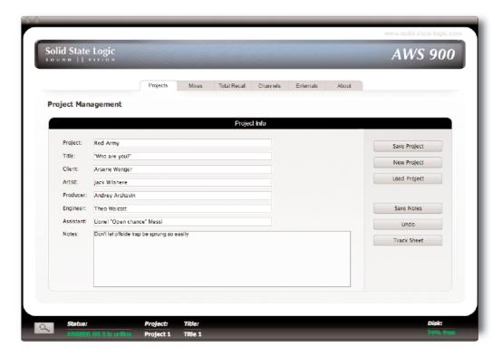
The first time you run the software the status bar will display the message 'No AWS Found, click on Find' in red. If the Remote cannot find the console it usually connects to, it will display 'AWS 900 SN XXXXX is offline'.
