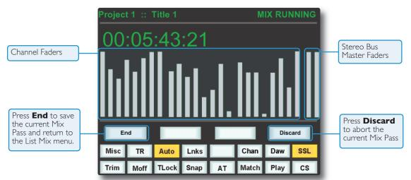
The system saves a Global Static reference mix of the fader levels and cut status at their positions when the **Execute** key is pressed. This is useful because it allows you to locate before the start of the mix and recover your original levels (i.e. reference mix). Also, if you are writing automation in a section that had no previous mix data, when you drop out of write the faders go back to their original levels.
