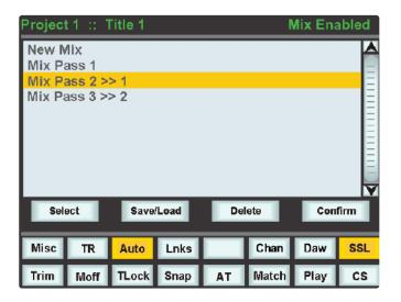
Now press the encoder switch or the **Select** soft key to select the New Mix Setup page.
