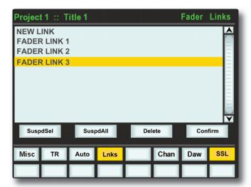
To set up a new Link, scroll to **New Link** and press the V-pot push switch. This will create a new entry in the list suffixed with a number. This entry will be automatically highlighted and faders can be added (or removed from the Link) by pressing the fader auto switch. Link numbers are shown in the scribble strip above the fader and the read fader status LEDS will indicate the faders in the currently selected Link.
