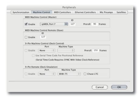
Enable MIDI Machine Control and select the Port on the MIDI Interface that is connected to AWS Port 4 MIDI IN or IP MIDI Port 7. Leave the ID as 127 (this sends to all connected devices). Open the Operation tab in Setup/Preferences:
