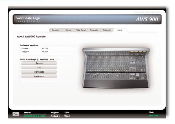
The **About** tab shows the current software versions of both console and browser and provides links to the SSL Support, FAQ's, Downloads and Registration areas of the SSL website.
