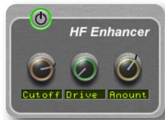
This process is not possible with a standard EQ, as instead of raising the relative level of a set of frequencies, it is adding harmonics to those frequencies therefore producing a more pleasing effect.
