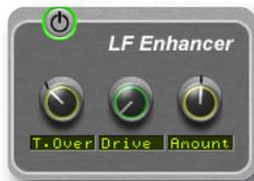
The incoming signal is low-pass filtered, harmonically enriched using the **Drive** control and added to the unprocessed signal using the **Amount** control.
