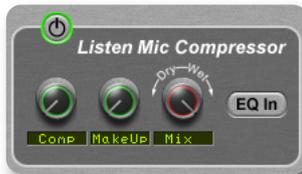
It now features the familiar Listen Mic Compressor sound, but with the option of EQ by-pass, offering full range compressor action. The addition of a **Mix** control gives the option to mix the compressed sound in with the uncompressed sound to taste, providing parallel or upwards compression.
