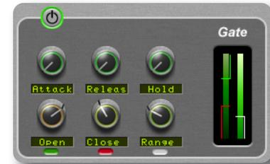
The Drumstrip gate provides six controls, a process In/Out button and a comprehensive multi-function meter.
