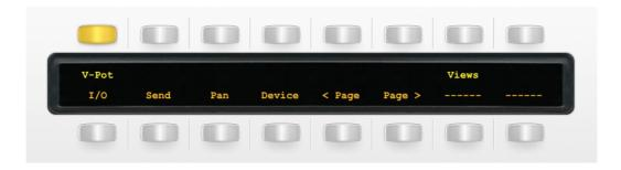
The first four keys, I/O, Send, Pan and Device determine what function the V-Pots are controlling.
